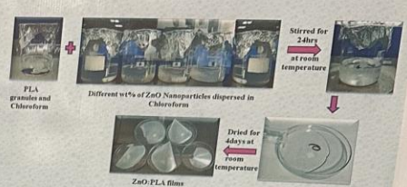
Fig 3: Graphical representation of fabrication of ZnO:PLA film by solution casting method
